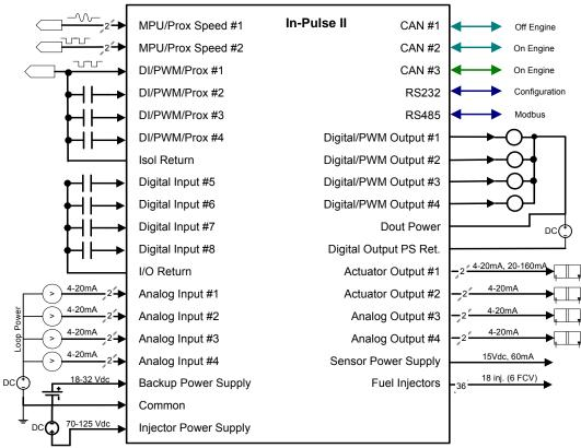
In-Pulse II Control Block Diagram
